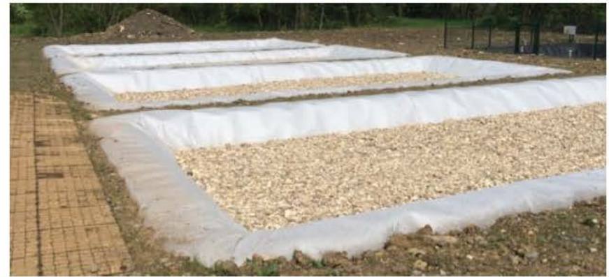
Lysimeter plots : pedogenesis and treatment of Technosols ( in situ chemical oxidation, soil construction, phytoremediation, natural attenuation, agromine)
